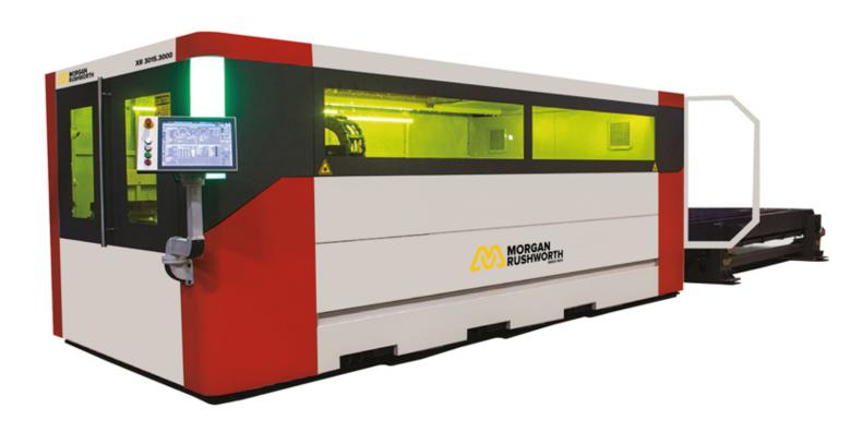
The Morgan Rushworth XS range of fibre lasers are available in a range of bed sizes and are equipped with an automatic shuttle table with dual pallet changer enabling parts to be safely loaded and unloaded whilst the machine is still cutting. Class leading components ensure superior cut quality, high reliability and reduced down time.
