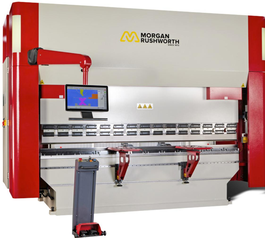
The Morgan Rushworth XPH range of hybrid press brakes are designed with an individual electro-hydraulic servo drive system for each of the left and right cylinders. With this system the hydraulics run on demand when the foot pedal is activated, rather than having a pump running continuously. This results in lower energy usage than a standard hydraulic machine as well as faster cycle times and extremely high accuracy.
