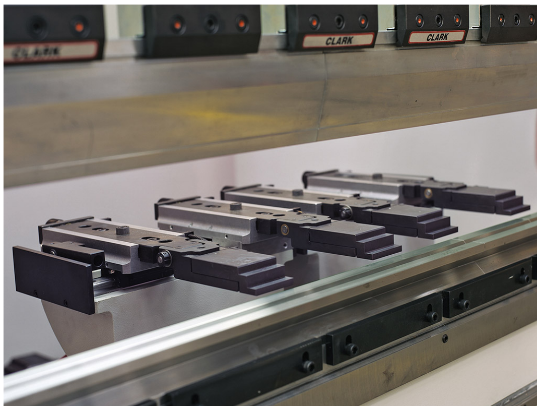
Optional Additional Back Gauge Fingers
