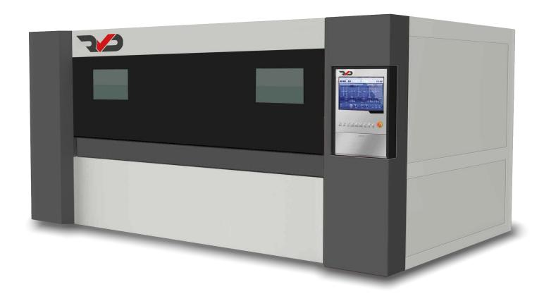
The RVD SmartFibre ER <u>fibre laser cutting machines</u> feature a compact design with a pull out cutting table in place of the shuttle table commonly used on many lasers. This space saving layout reduces the machine's footprint by 50% when compared to equivalent shuttle table models, while still allowing for easy loading and unloading outside of the cutting enclosure.
