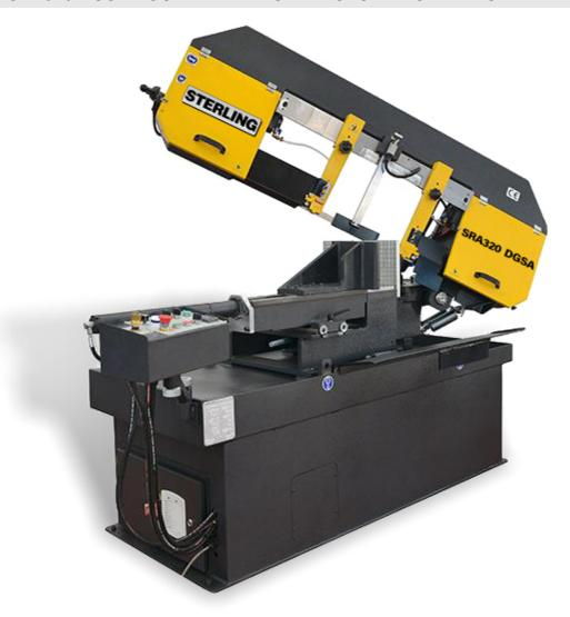
The Sterling SRA320 DGSA band saw is a double mitring model, with generous beam and tube capacities. This model features hydraulic clamping and hydraulic bow down feed with automatic bow height return. Mitre angle is set using a digital angle display and the saw also features variable cutting speed to work with a range of material. A 34mm blade width is standard which allows the cutting of heavier sections without the loss of accuracy.
