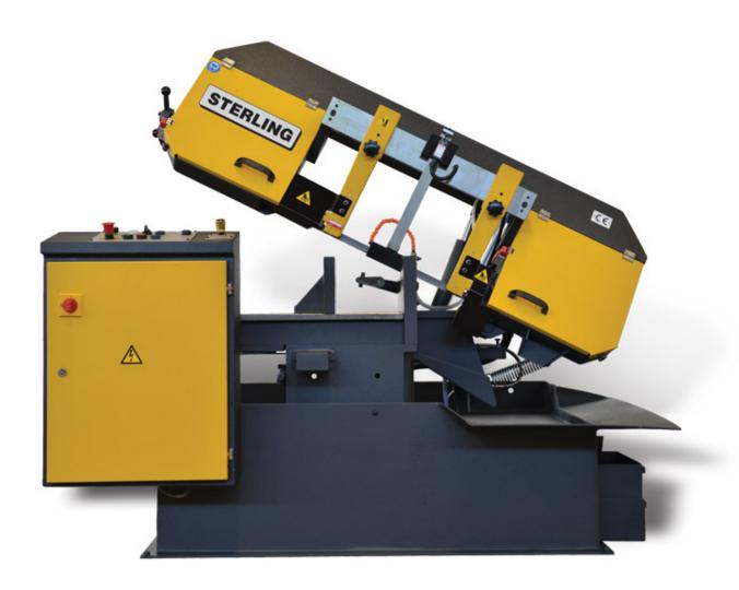
The Sterling SRA320 GSA and GSAL semi-automatic models feature a single mitring head design with the ability to mitre up to 60 degrees. The SRA320 GSAL with its long bow design not only caters for up to 610mm maximum cutting width at 90 degrees but also benefits from the ability to still cut tube of up to 320mm diameter at a 45 degree mitre.
