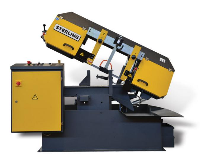
The Sterling SRA320 GSAL semi-automatic model features a single mitring head design with the ability to mitre up to 60 degrees. With its long bow design, it not only caters for up to 610mm maximum cutting width at 90 degrees, but also benefits from the ability to cut tube of up to 320mm diameter at a 45 degree mitre.
