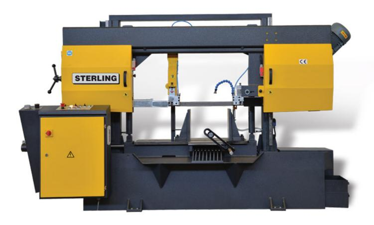
The Sterling twin column band saw models begin with a wide range of semi-automatic models in capacities from 325mm to a massive 1300mm tube cutting capacity. With this extremely rigid twin column design, the bow travels on precision linear guides offering exceptional precision in the cut. All models feature hydraulic vices, hydraulic downfeed and bow return as standard. Infinitely variable blade speed allows the cutting of a wide range of material types, including more exotic materials.
