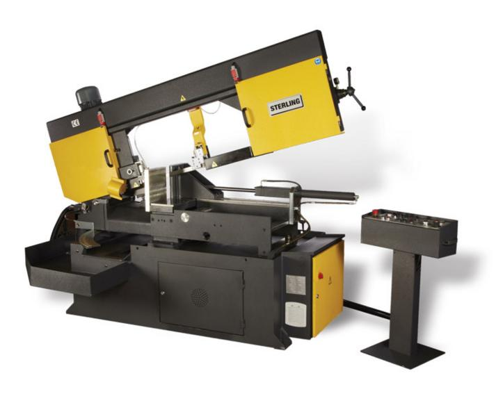
The Sterling SRA360 DGSA and SRA440 DGSA band saws are large capacity double mitring head models, featuring five hydraulic systems for ultimate productivity. Vice clamping, bow downfeed, bow return, bow counter balancing, and mitre setting at any angle are all performed using hydraulics for superior performance and ease of use.
